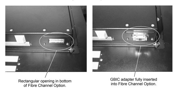
Figure 4-12 Inserting GBIC Adapter into Fibre Channel Option
